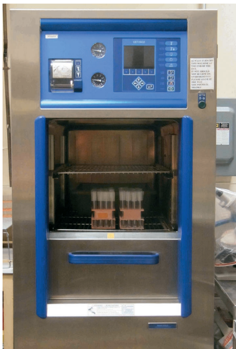
Figure 1.2 Autoclaves use steam under pressure to sterilize biohazardous materials prior to disposal. ©Barry Chess
